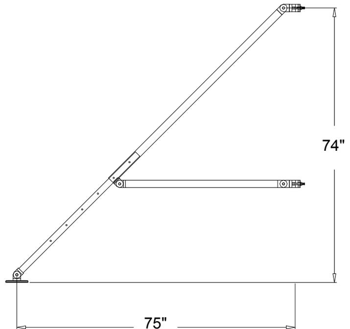
The ground support tower system can be used outside but must be suitably anchored from the top of each tower sleeve block to the ground via a guy wire to a suitable ground anchor. We recommend that the bases are sat on top of a 3' square piece of 3/4" plywood. Should a cover be required please refer to James Thomas Engineering for an approved design to suit your requirements.
