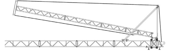
The ground support tower system can be used outside but must be suitably anchored from the top of each tower sleeve block to the ground via a guy wire to a suitable ground anchor. We recommend that the bases are placed on top of a 3' square piece of 3/4" plywood. Should a cover be required, please refer to James Thomas Engineering for an approved design to suit your requirements.
