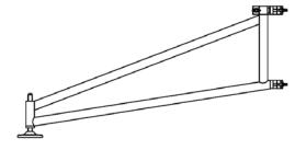
**Outrigger arms** are required when using less than 3 towers. These are designed to provide stability and rigidity to single or 2 tower systems.
